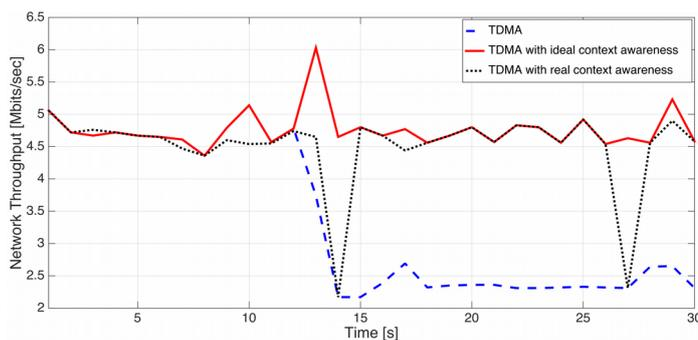
Figure 4: Throughput comparison for TDMA
